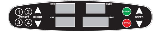
The LED window shows: MPH (speed), TIME, MILES (distance) and CAL. (calories).
