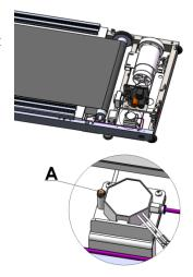
4. Reinstall the motor cover and tighten screws.
