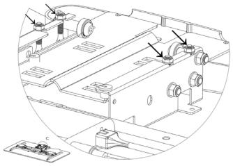
**Step3:** Connect the treadmill and table control wires and place the emergency switch onto the console.
