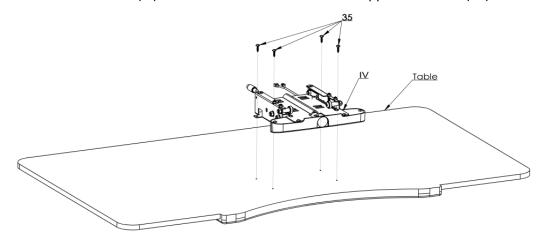
Remarks: Adjust the tension of the console set on the rails by the 4 pieces of screws as the arrows point in the below picture.
